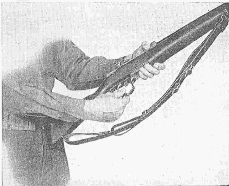
PLATE 4. REMOVING TRIGGER HOUSING GROUP
