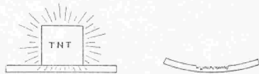
FIGURE 33. General cavitation effect with solid block of explosive, which leads to discovery of the "Munroe effect" (shape charge).
