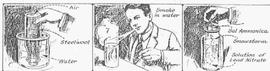
The drawing at the left illustrates an experiment for producing vacuum by rusting iron. Center, a solution of hypo becomes milky when cigarette smoke is blown upon it. Sal ammoniac will produce a very gentle, pretty snowstorm if the directions given in Mr. Wailes' article are followed.
