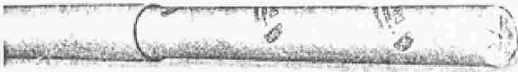
FIGURE 21. Dynamite cartridge with marriage or joining tube. (Courtesy E. I. Du Pont de Nemours Co.)
