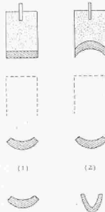
FIGURE 38. Misnay-Schardin effect (plate charge). 1) Flat plate, 2) Concave plate.
