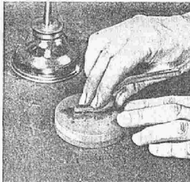
After filing, teeth are evened by rubbing on an oilstone. A final bit of filing may be in order, to sharpen teeth that were too long
