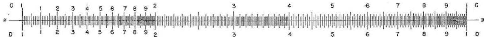
FIG. 1-14. Typical Slide Rule Scales. (The second one may be cut out and pasted on cardboard or wood to make a model slide rule. Also cut along line x-y .)
