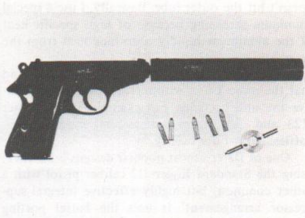
The Dater "James Bond Special," a model R22-SL internally threaded into a .22 Walther PPK-S.
