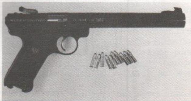
Phil Dater's highly respected RST sound suppressor on a Ruger RST-4 pistol. The Dater modification uses adjustable sights.
