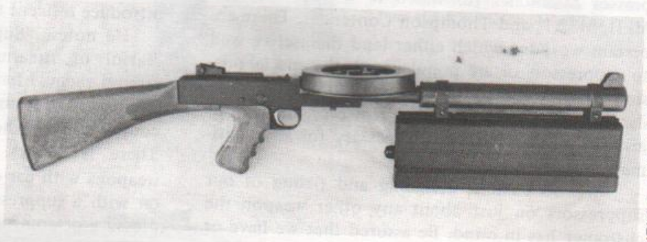
American 180 suppressor/barrel assembly with laser sight mounted.
