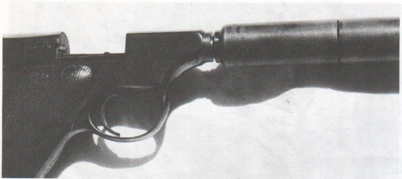
Side view of the .22 caliber Woodsman with the Gold Spot suppressor in place.
