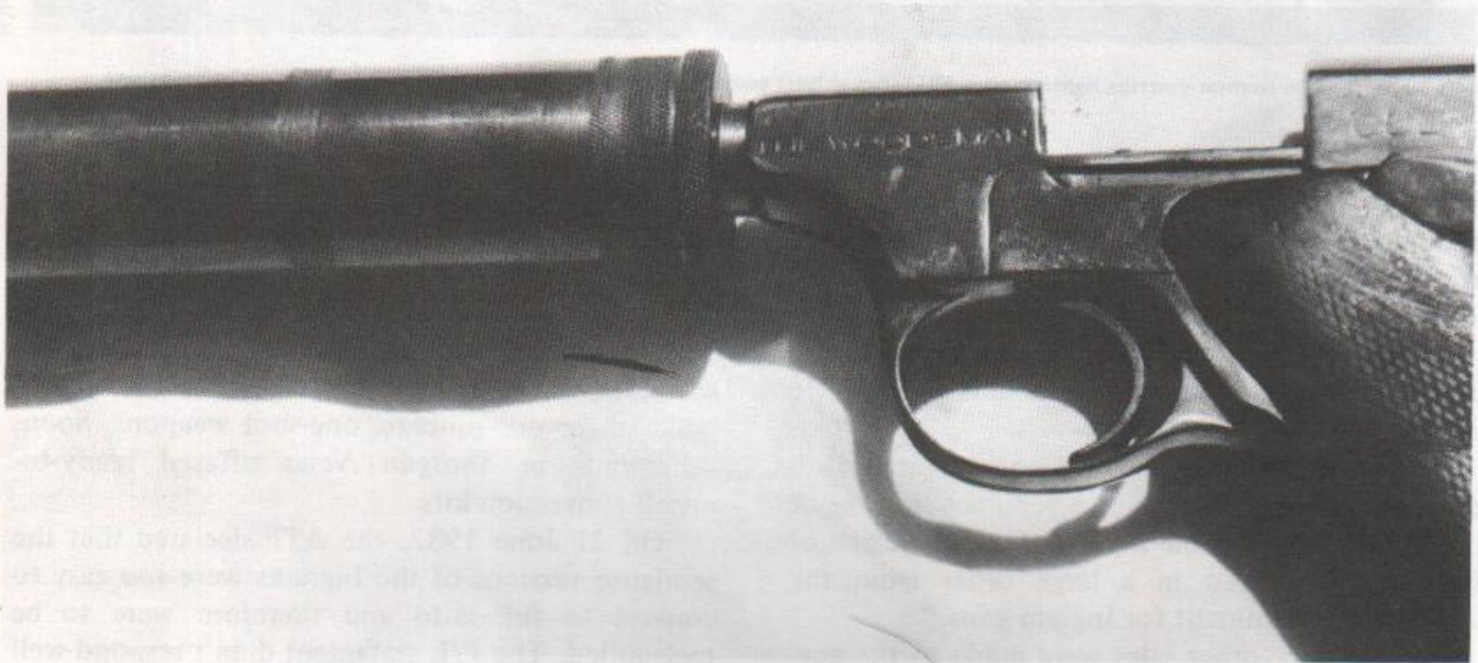
Side view of the Colt Woodsman, .22, with a homebuilt suppressor from Australia, where possession of such units is quasi-illegal. Few arrests are made, however.
