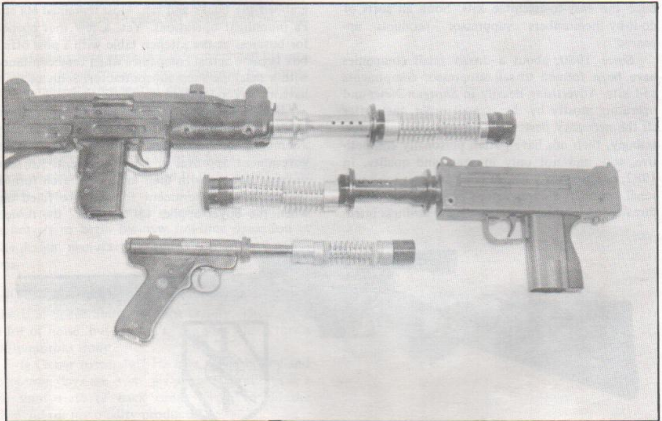
R. F. P.'s Uzi kit, the MAC 10 kit, and the Ruger RST 4 kit. Their Uzi design is unique in that the suppressor kit slides over the short barrel, replacing the barrel nut, which keeps the overall length to a minimum.
