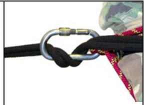
Figure 10-32. SEAT HIP RAPPEL WITH CARABINER WRAP DESCENDER
