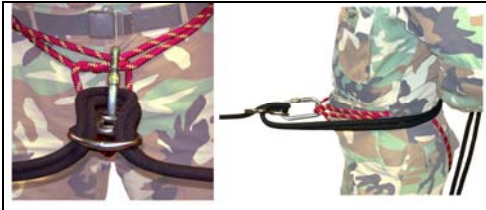
Figure 10-32. SEAT HIP RAPPEL WITH CARABINER WRAP DESCENDER
