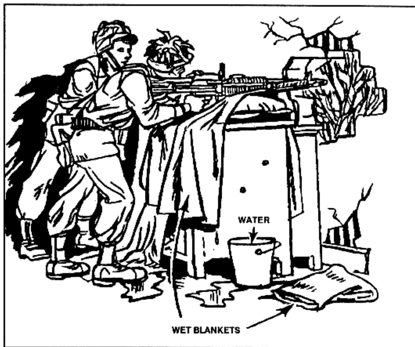
Figure 5-46. Wet blanket used to keep dust down.
