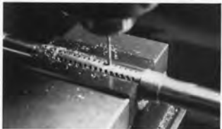
Ports are drilled in the barrel using the milling machine.
