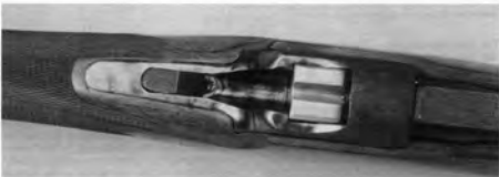
Falling block action with square breechblock.
