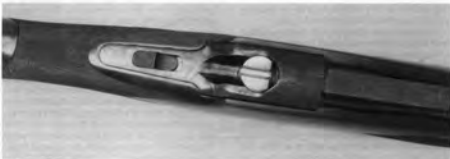
Falling-block action with round breechblock.
