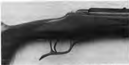
A joint pattern of "recessed" or "lost" checkering whereby the area to be checkered is recessed or cut away to a predetermined depth before the checkering is done. This is not really worth the extra effort involved.
