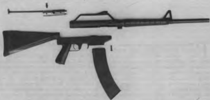
Inertia-locked autoloading blowback action.
