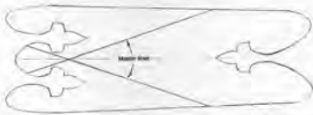
Fleur-de-lis wraparound forward pattern. Dimensions must be changed to conform to individual stocks.
