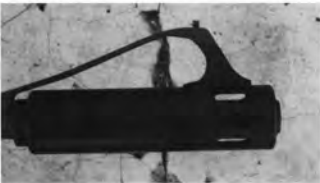
Threaded arbor is mounted in lathe chuck. The brake is screwed onto it for outside finish cuts.
