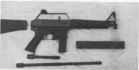
A 9mm conversion unit on an AR-15/M16 lower receiver shown with a detachable butt stock; 15-, 10- (mounted), and 6-inch barrels; and 15- and 30-round magazines. Using an original M16 receiver to make a 6-inch-barrel pistol is making a "short-barreled rifle" according to the BATF.
