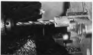
The pilot hole is drilled through the brake body.
