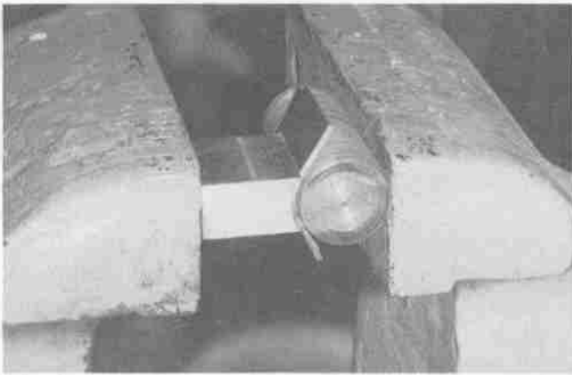
Vise jaws are drawn together, forming curve on bottom.
