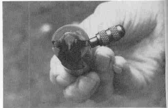
Open-bolt assembly; fixed firing pin is on lower side of bolt face.
