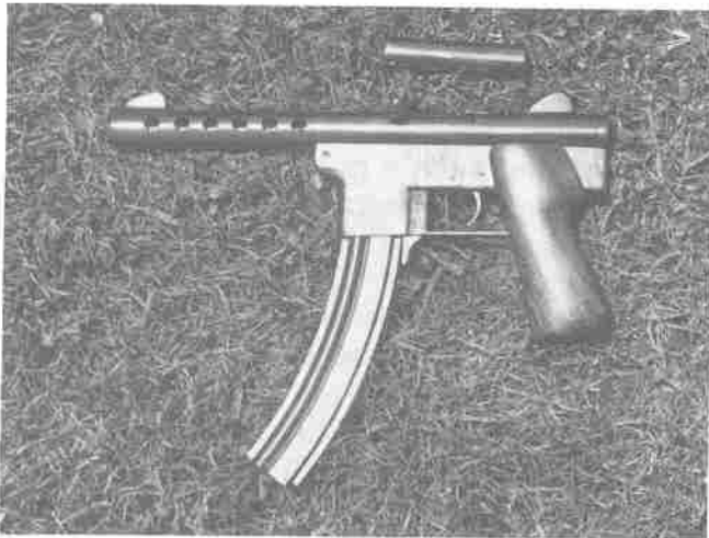
The open-bolt assembly shown just above the gun is interchangeable with the closed bolt.
