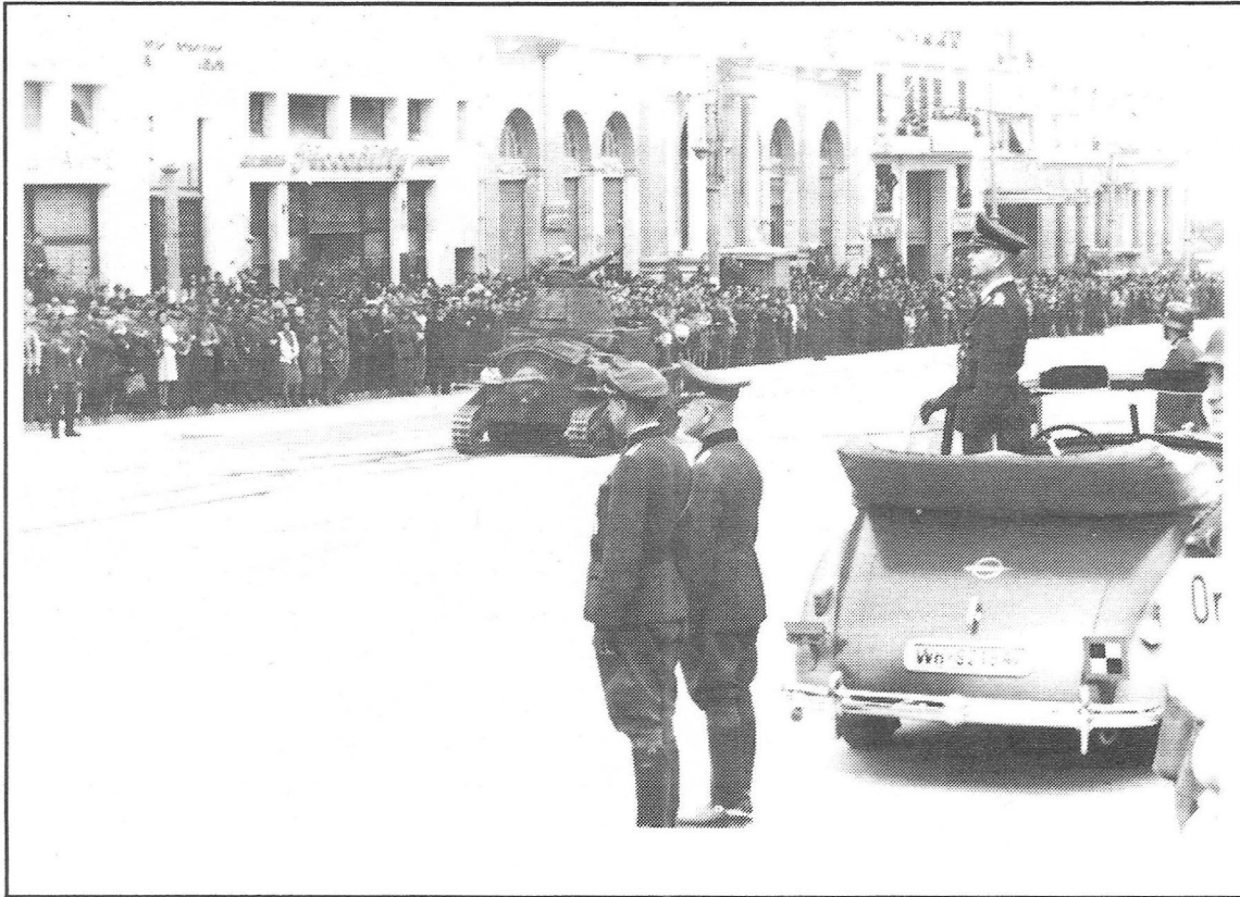
ABOVE: Parade of the German Police, somewhere in a large Greek city, late 1943. The vehicle in the street appears to be a captured Italian L.6 (carrying a 37mm cannon). The Germans used captured Italian equipment (after Italy left the war) as often as possible, and in particular, supplied their Order Police and auxiliary forces with these and other foreign weapons. This Italian vehicle has been put to use by the German Order Police. A close examination of the rear vehicle license plate, under a magnifying glass revealed that indeed the German Police had put it to use. Bundesarchiv.
