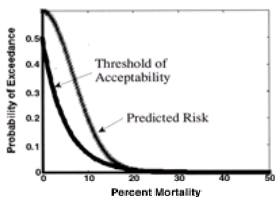
Figure 29-7. Illustration of risk manager's threshold of acceptability (shaded line) and predicted risk from a simulation model (data points).
