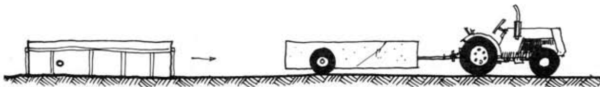
FIGURE 12.26 ICE TOWED AS A BUGGY. Ice forms in moulds can be easily moved to cool stores.
