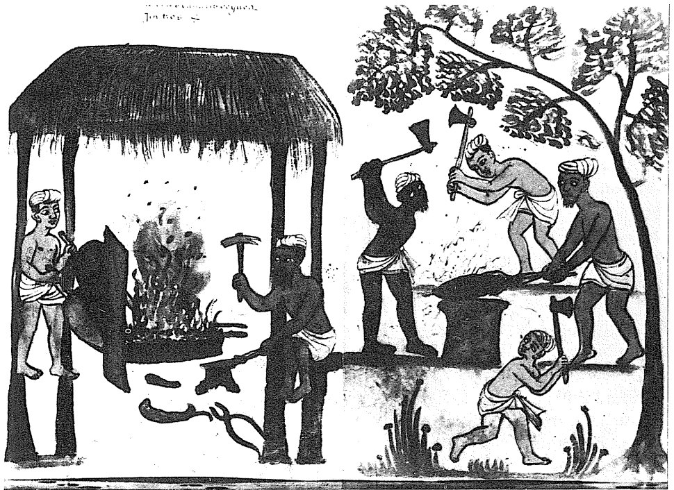
Native blacksmiths in sixteenth-century Goa: note the elementary technology, with hand bellows and the peculiar hammers which look as if they might also be used as axes. (Photo F. Quilici.)
