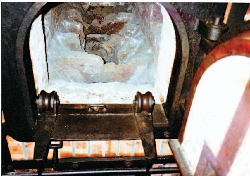
Document 40: Crematorium of Buchenwald. Topf triple-muffle coke-fired oven. Central muffle. Roller-device for coffin introduction cart ( Sargeinführungswagen ) in position for operation. © Carlo Mattogno.
