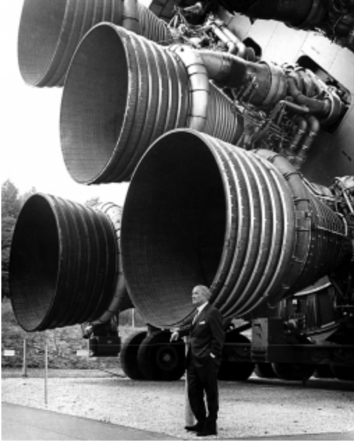
Werner Von Braun with the F-1 engines of the Saturn V first stage rocket he invented, which took men to the moon, at the U.S. Space and Rocket Center.
