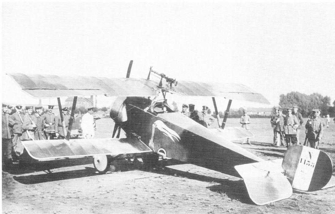
The Nieuport 11, a captured example of which is seen here, had no synchronisation gear and relied on firing over the propeller arc, which was not as efficient as the Fokker Eindecker it faced.
