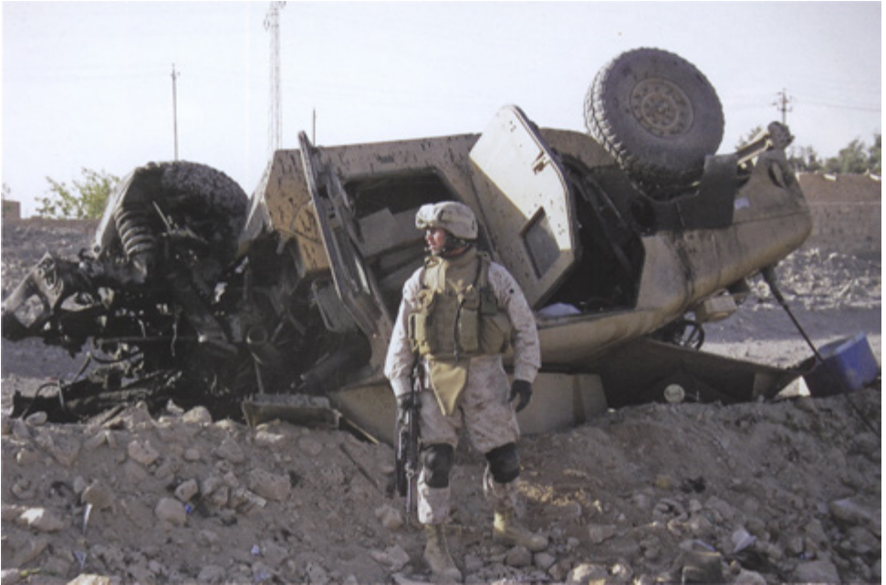
Concealed IEDs utilizing artillery shells in Iraq and Afghanistan were detonated by remote control directly underneath patrol vehicles and produced multiple penetration and blast injuries. (USMC)
