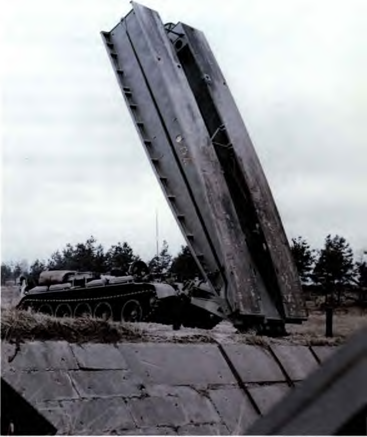
A bridge-laying armoured vehicle prepares to lay a 10m
