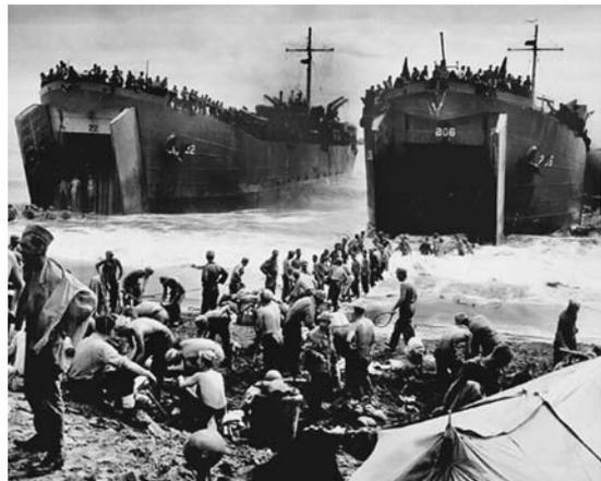
LSTs (Landing Ships, Tank) disgorge men and equipment on a Pacific island. These large ships were intended to deliver men directly from sea to shore—without the dangers of transfer to and disembarkation from small landing craft. (U.S. Navy)
