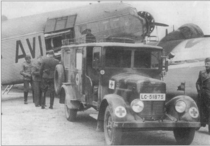
A Phänomen Granit 25H ambulance of San88 carries Condor Legion wounded to a Ju 52 for evacuation to Germany. Note the ambulance's number plate with the initials 'LC-', and the aircraft's civil livery. (Campesino)
