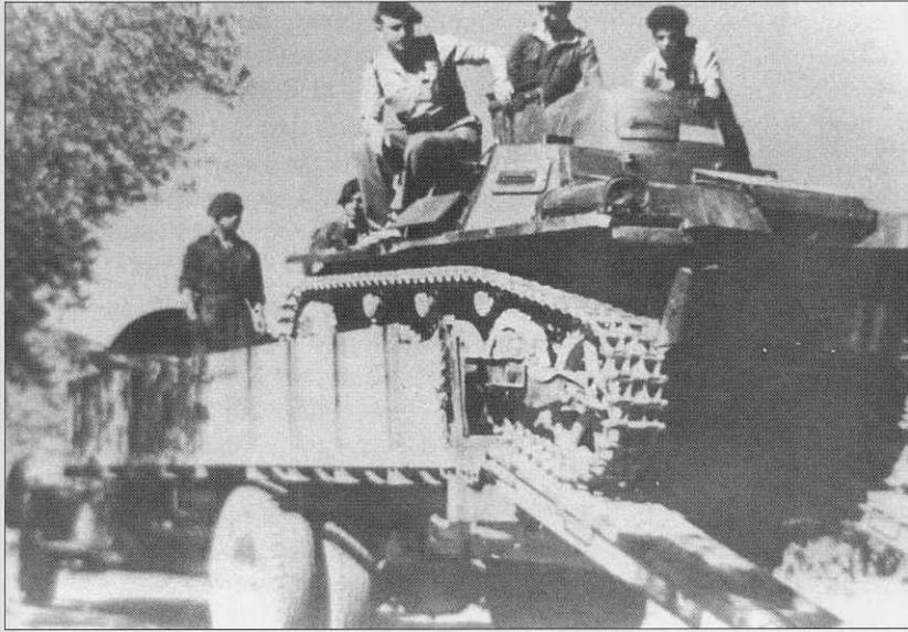
Panzer I of a Spanish unit being driven on to a truck, probably an American GMC ACX-504. The Transport Company of Panzergruppe Drohne had the much larger Vomag DL48 trucks towing SdAh 115 transport trailers. (Steven Zaloga)
