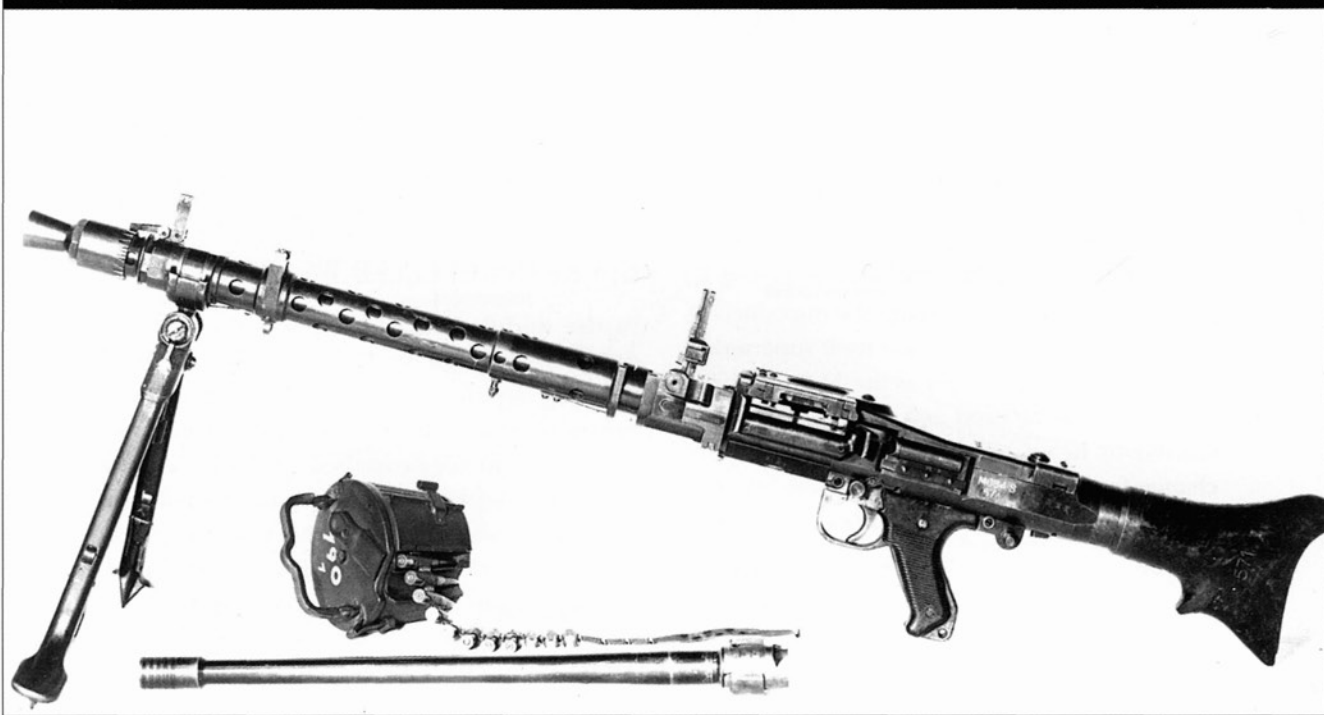
The standard machine gun, the MG 34. It is shown here mounted on a tripod in its heavy machine gun mode and on a bipod in light machine gun mode.
