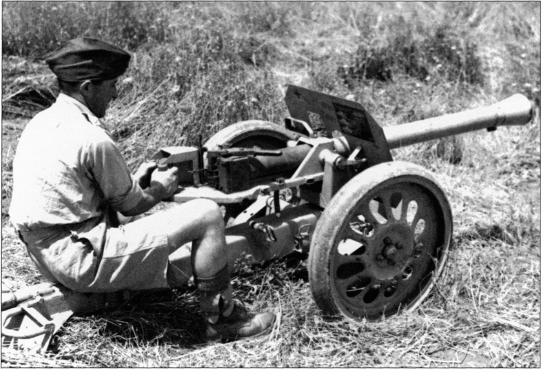
The improvement on the Panzerschreck was a wheeled version known as the 'Püppchen'. It is seen in this photograph being operated by a British soldier.
