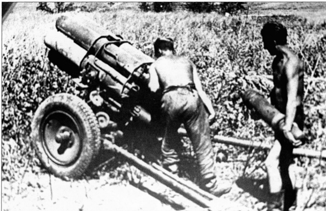
The Nebelwerfer was a very effective weapon when used against infantry. It fired a pattern of six projectiles which screamed through the air, creating a nerve-shattering noise. Here the shells are being loaded into the barrels, from which they would be fired by electrical charge. Their discharge was accompanied by huge trails of fire and smoke.
