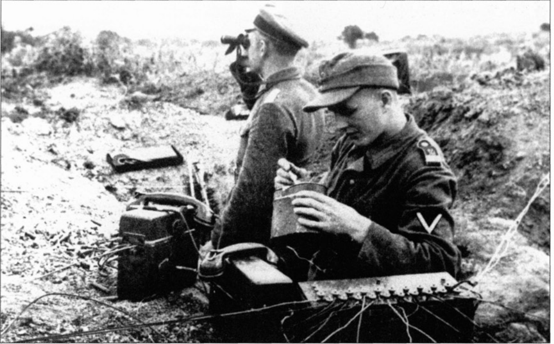
An advanced outpost of the 'Großdeutschland' Division, showing the field telephone exchange (the ten-line exchange).
