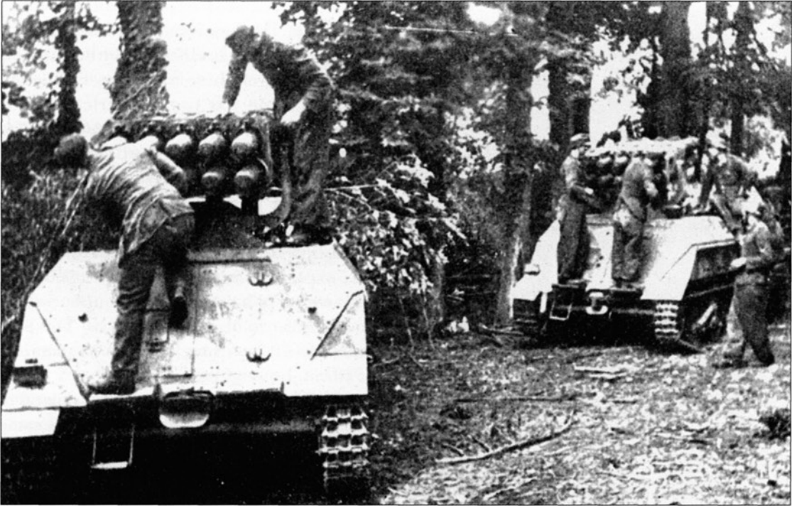
The Panzerwerfer 42 was a motorized and upgunned version of the standard Nebelwerfer. Here, the ten 15 cm tubes of the Panzerwerfer 42 are being loaded.
