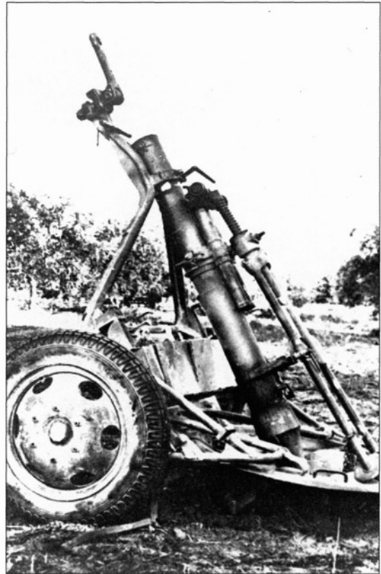
The 120 mm mortar, here shown mounted on its wheeled carriage.
