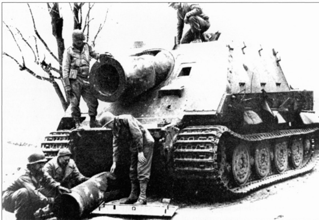
The 65-tonne Sturm Tiger carried a 38 cm mortar whose projectile exploded with devastating effect. Only ten Sturm Tigers were brought into service, and these were formed into two companies. One company fought in Warsaw, and the second in the Battle of the Bulge, December 1944.
