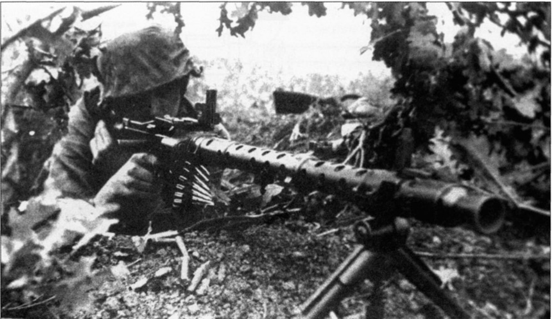
The standard machine gun, with which the German forces entered the Second World War, was the MG 34, seen here in its light machine gun mode on a bipod.
