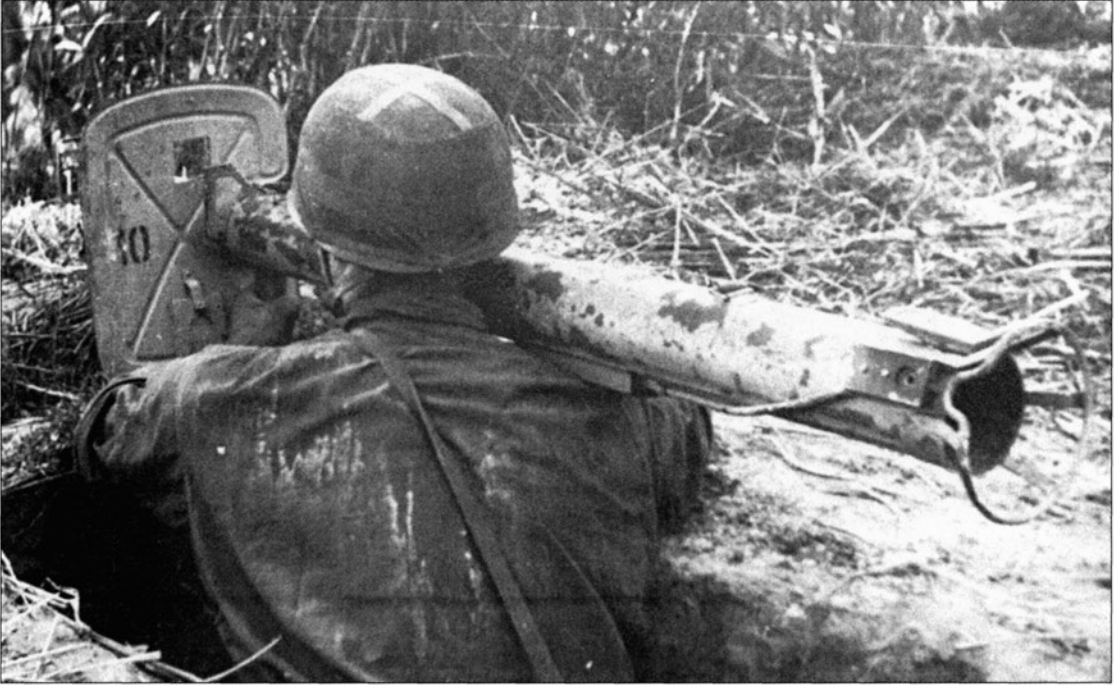
A German paratrooper ready to fire the Panzerschreck anti-tank rocket launcher. This is the later version of the weapon, for it has an observation panel in the protective shield.
