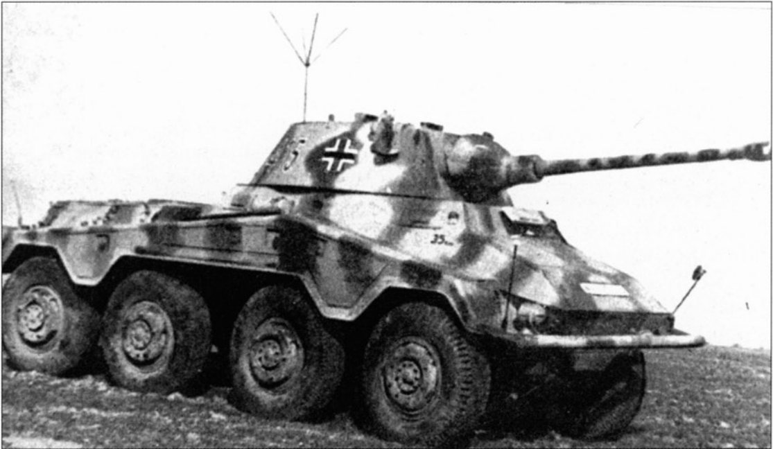
The second variant of the Sd Kfz series, the 234/2, also known as the Puma, carried a 5 cm gun in a rotating turret.
