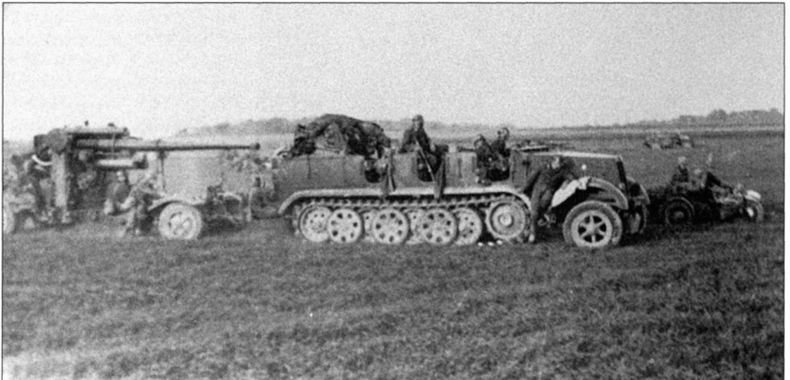
The weapons of the German Field Artillery included several which had been introduced as anti-aircraft guns but which were found to be particularly effective as anti-tank guns. This picture shows an 88 mm gun being towed into action behind a half-track vehicle.
