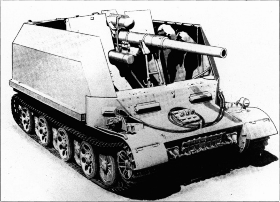
This drawing is of the Krupp's prototype for a self-propelled gun mounting an 88 mm weapon.
