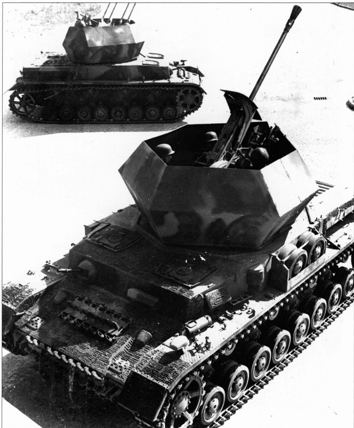
From the middle years of the war, Panzer divisions needed anti-aircraft protection. This picture shows two such flak Panzers. In the foreground is the Ostwind ('East Wind'), mounting a 3.7 cm gun on a Panzer IV chassis. In the background is the Wirbelwind ('Whirlwind'), which carried four flak guns of 2 cm calibre.
