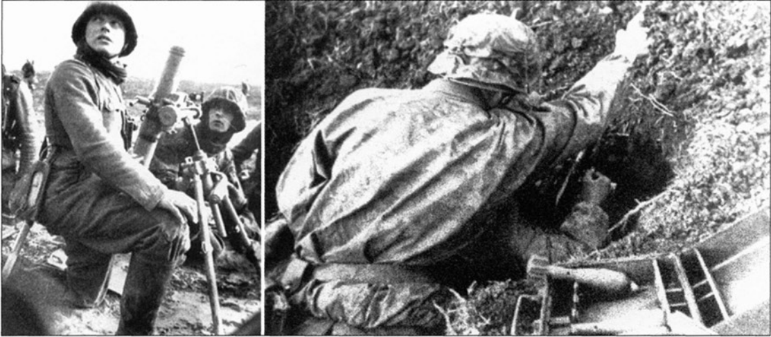
The two mortars on standard issue to German infantry units. On the left, the 81 mm piece which fired its bomb from a fixed firing pin, and on the right, the 50 mm mortar, which was operated by a wheel which activated a firing pin.
