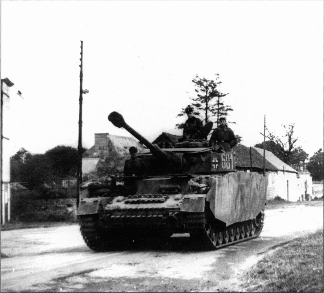
The Panzer IV shown in this photograph carries armoured plate skirts to protect the tracks against hollow-charge anti-tank projectiles.
