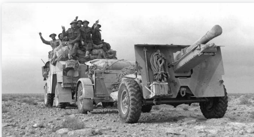
A British artillery tractor pulls a limber and gun across the desert ready for the next battle. The crew of the 25-pdr field gun ride on top of their stores and kit on the outside of the Morris C8 4 x 4 Quad. (IWM, E7245)
