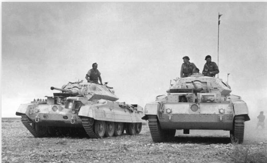
Two Crusader cruiser tanks move forwards during the operation. This picture was taken on 26 November at the height of the tank battles around Sidi Rezegh. The Crusader's main 2-pdr weapon seems tiny in comparison with those found on German tanks. (IWM, E6724)
