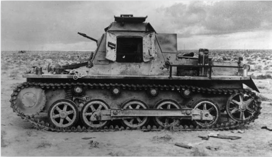
A Panzer I Ausf. B of Panzer-Regiment 5 knocked out and captured during Operation Crusader . By this time in the war the Panzer I was obsolete and only a few were shipped to North Africa in the early days of the Afrika Korps. (IWM, E7074)
