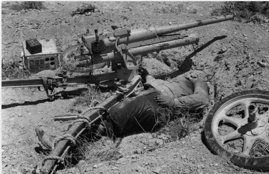
A knocked-out Italian Cannone da 47/32 M35 anti-tank gun with one of its crew lying dead beside it. (IWM, E13485)
