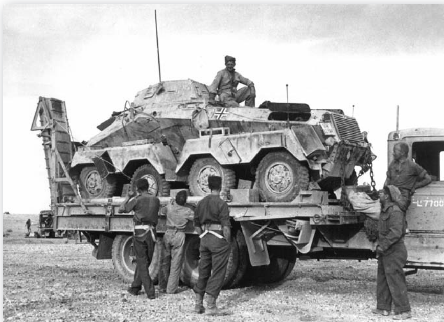
A captured Panzerspähwagen SdKfz 231 eight-wheel armoured car is loaded onto a tank conveyor, just after the start of the Crusader battle. These heavy reconnaissance vehicles, armed with a 20mm cannon, were held in a position of awe by the crews of their British counterparts in view of their size and power. IWM, 6710
