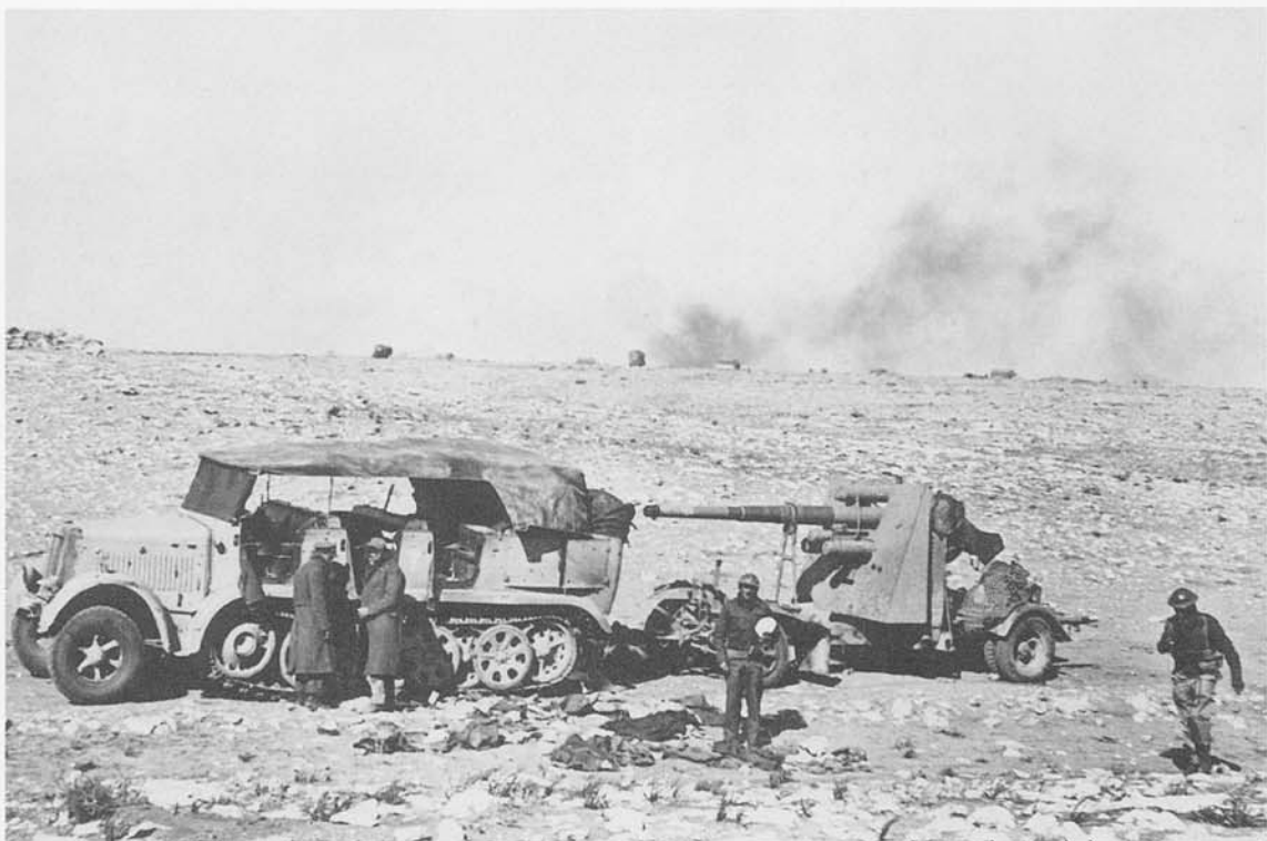
Probably the most feared anti-tank gun in the desert was the German 8.8cm AA/anti-tank gun, seen here being towed by a Sd Kfz 251/7 halftrack. The dreaded '88' could easily penetrate any Allied tank at considerable distances. (IWM — MH 181)
