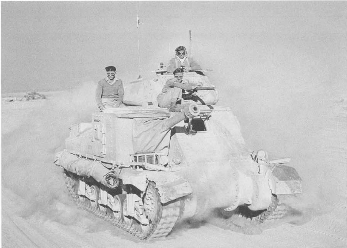
A Grant at speed. This was the American M3 medium tank, which was armed with a 75mm gun in a side sponson and a 37mm gun in the small turret on top. It created quite a stir when it first came into service in the desert. (IWM – E 18684)
