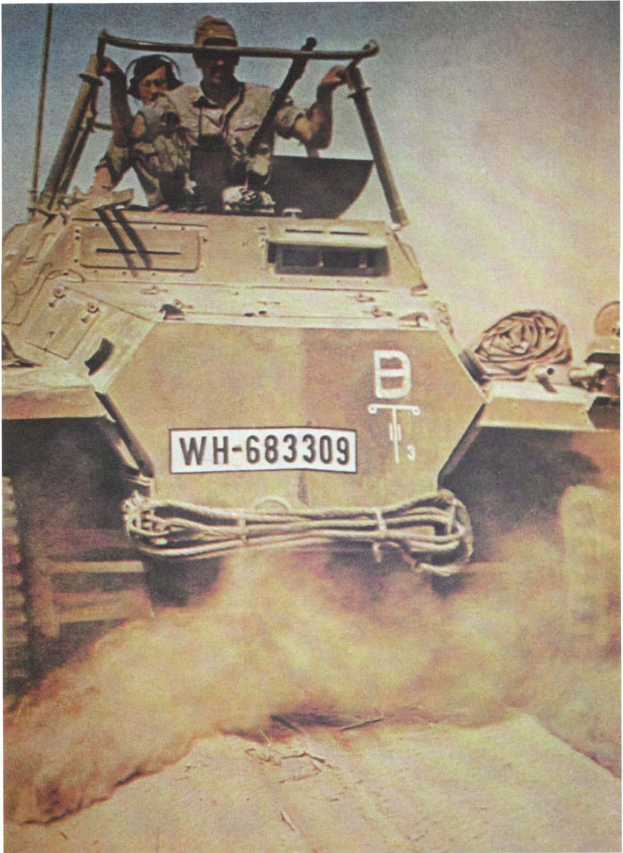
A German SdKfz 250/3 lichter Funkpanzerwagen (light radio vehicle) belonging to 21st Panzer Division. The sign below the divisional tactical sign represents a towed artillery unit. (Signal via Author's Collection)
