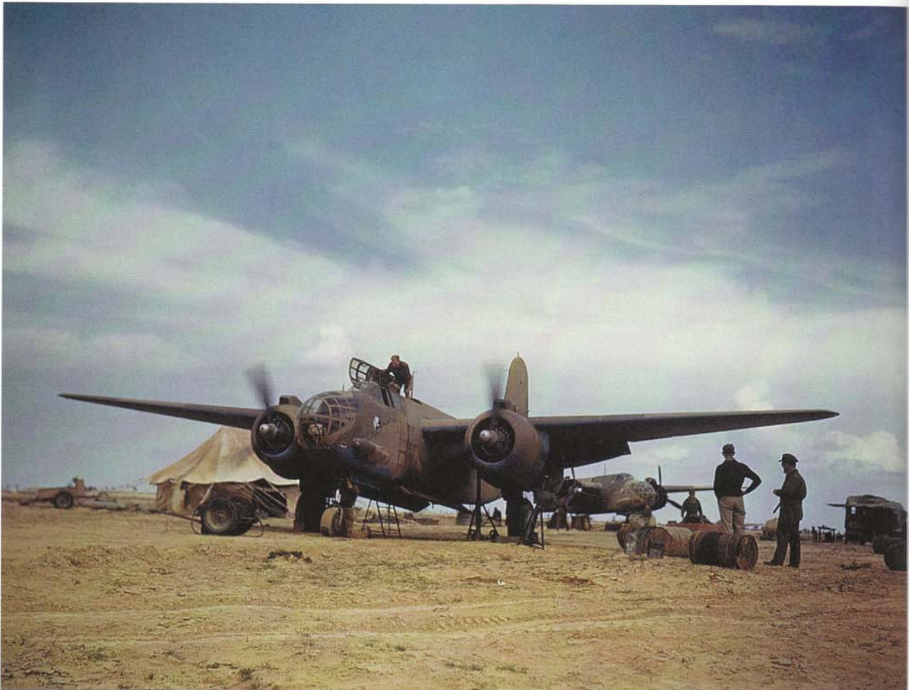
Running up the engines on a Douglas DB-7 Boston aircraft, belonging to 24 Squadron of the South African Air Force, May 1943. (IWM – TR 856)
