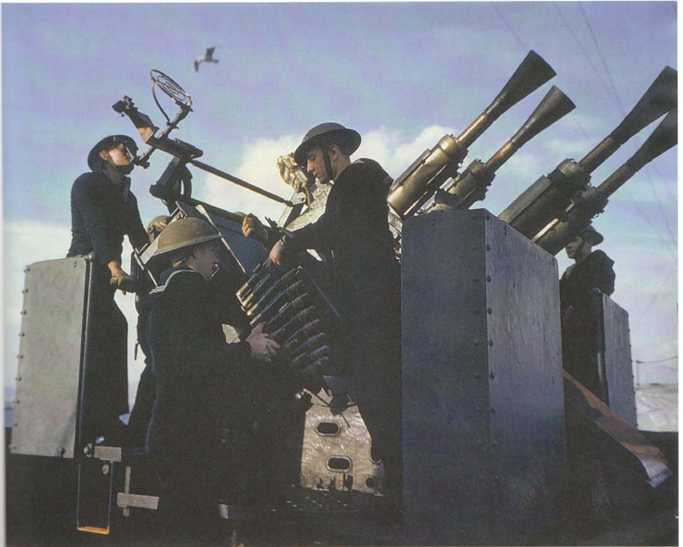
Firing the close-range AA pom-poms. These were 2pdr AA guns which could be fitted in single, four and eight barrel mountings. It was also known as the 'Chicago Piano'! (IWM - TR 1420)
