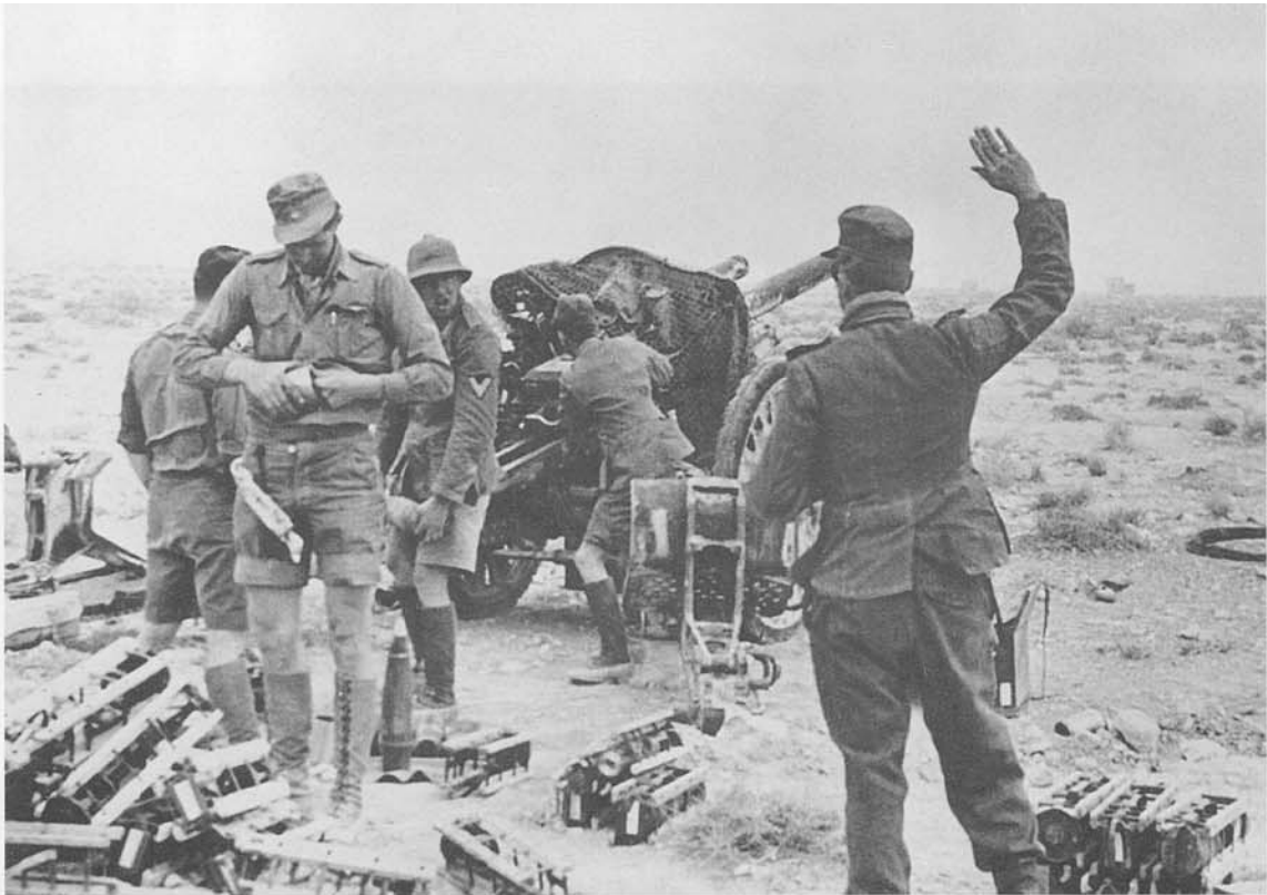
Heavy pounding. The 10.5cm le FH 18 was the standard light field howitzer used by the DAK. It was fitted with a muzzle brake when using more powerful propellant loads. (IWM — MH 5568)
