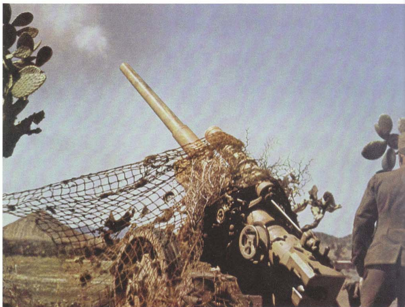
A German 10cm Kanone 18 medium field artillery piece in action in Tunisia. It was really a bit too heavy to be towed by horses, and its small shell weight (15.4kg) was disappointing. It was eventually relegated to coastal artillery. (IWM – TR 152)
