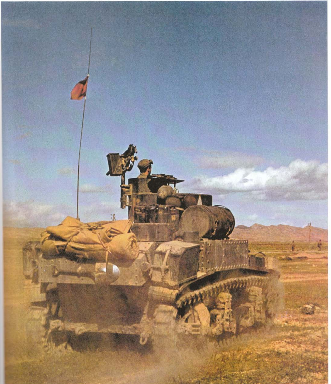
Well-Hoden US light tank moves across the desert. The Americans called them the M3 light tank series, the British named them 'Stuart', however, the British crews who were the first to use them in the desert just called the little tank 'Honey' because they were mechanically reliable and easy to crew. Weighing some 12.7 tons, the M3A1, for example, mounted a 37mm gun as its main armament and had a top speed of 36mph. (Time Life)
