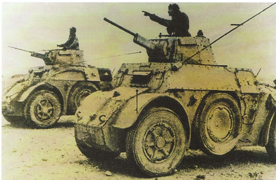
Two Italian Autoblinda AB 41 armoured cars on patrol in the desert. The main difference from the earlier AB 40 was the 20mm gun and coaxially mounted machine-gun in the turret in place of twin 8mm machine-guns. It was the most widely used Italian armoured car of the war. (Author's Collection)
