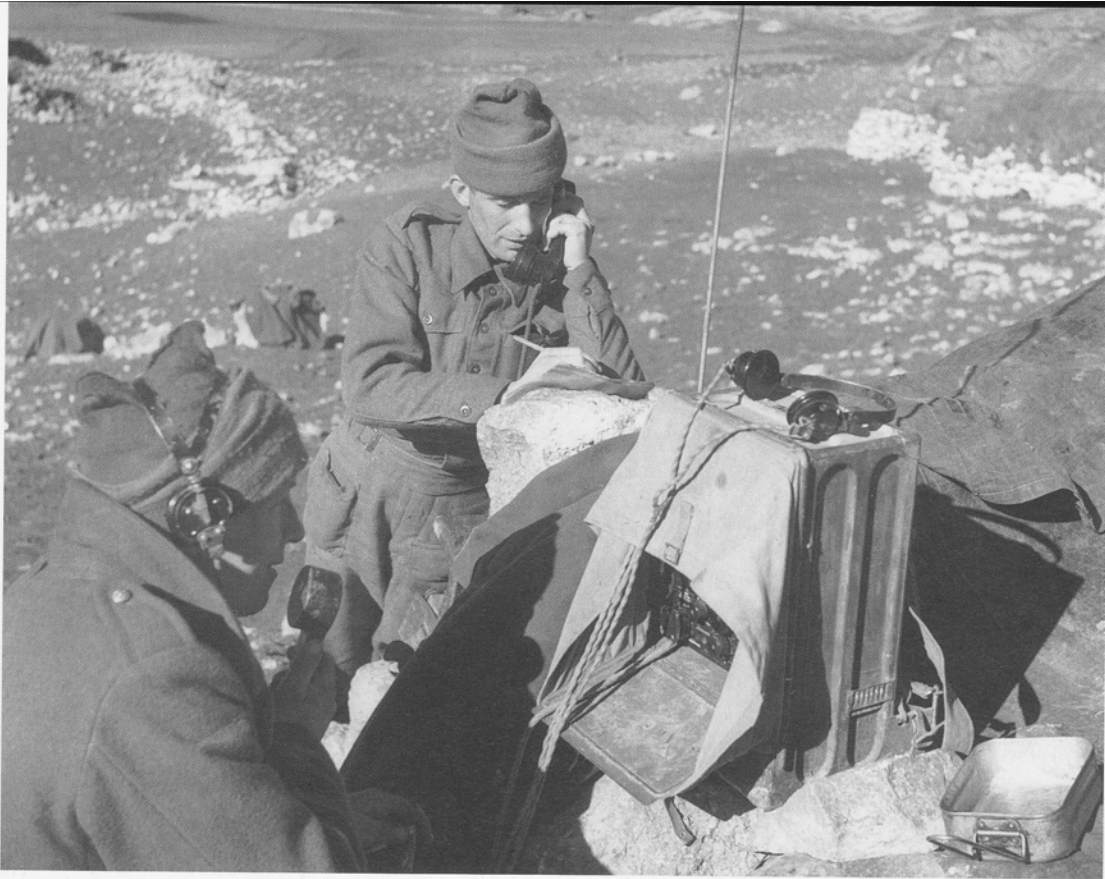
'Report my Signals, Over!' Good communications were vital in battle. Here infantry signallers use an 18 set, which was man-portable and designed to be used between Bn HQ and its sub-units. (IWM - NA 374)
