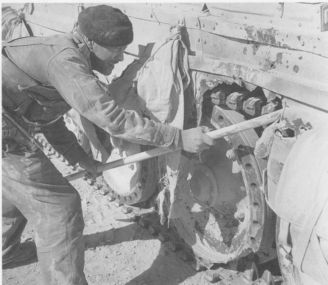
In defence tanks were often used static, firing from hull-down positions, but a proportion were always kept back for counter-attack purposes. Whatever their use, crews still had work to do. Here a crewman tries to prise twisted metal away from the track of his Crusader, after it has received a direct hit – fortunately not from a very powerful gun or it would have penetrated. (IWM – E 18690)
