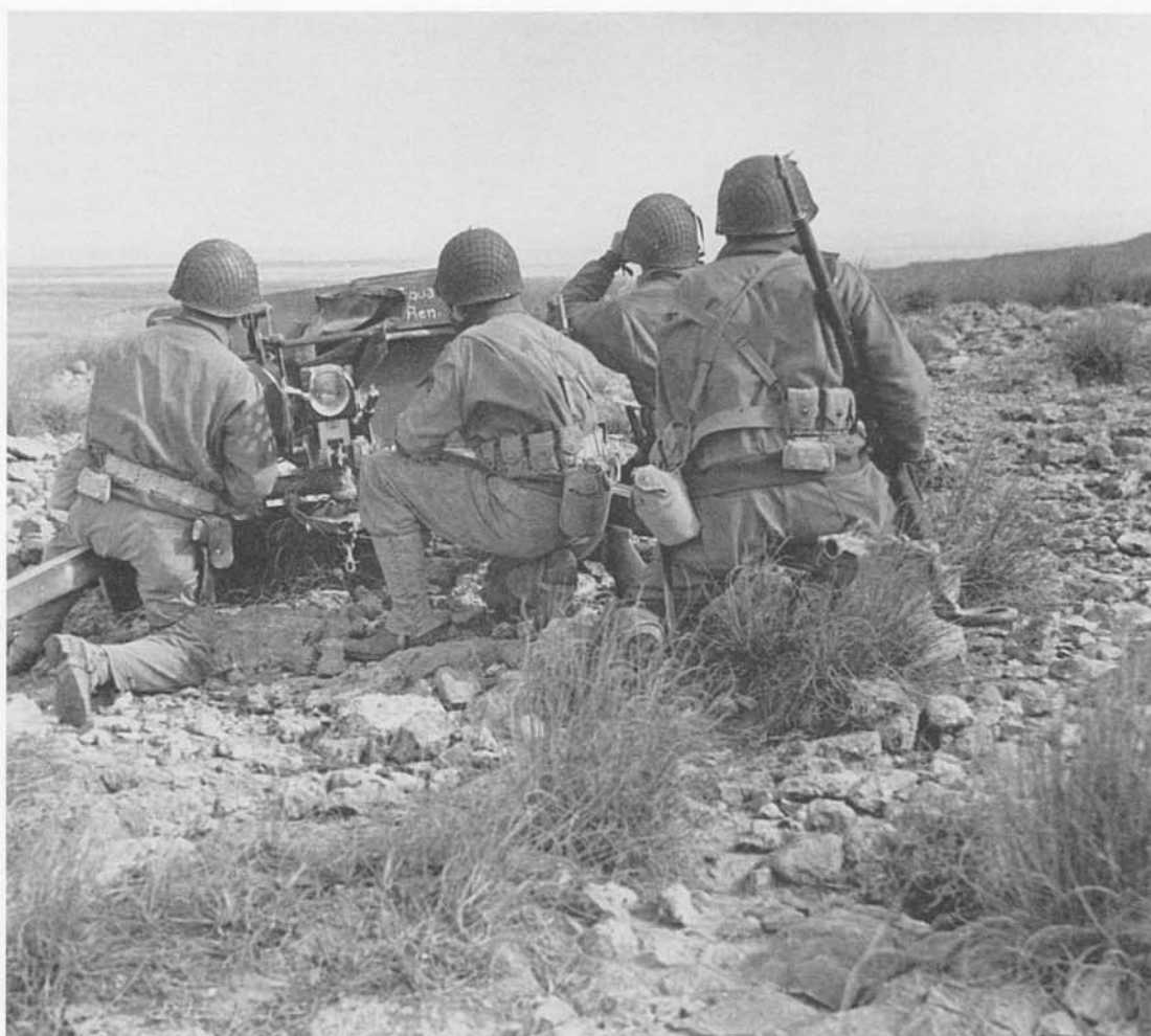
Close-up of an American gun crew manning their 37mm M3A1 anti-tank gun, which had a muzzle velocity of 2,900 ft/sec. Armour penetration using AP was only 1 inch at 1000 yards, but double that with APC ammunition. They have set up their gun to cover enemy tank approaches to Sidi Bou Zid. (Real War Photos - A 1152)
