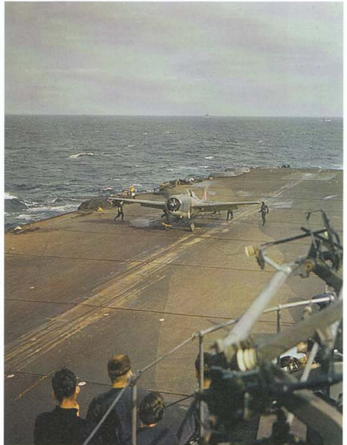
Excellent shot of a Grumman Wildcat on the flight deck of the aircraft carrier HMS Formidable , November 1942. One of the Illustrious class carriers, it could carry over sixty aircraft and was built in 1937. (IWM – TR 284)
