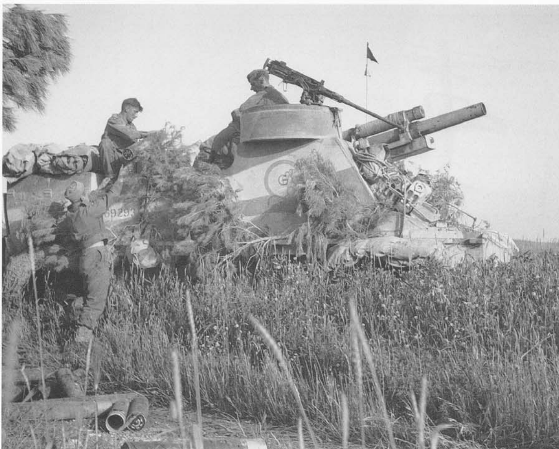
Operation 'Vulcan'. The Allies began their final push with elements of both armies. This SP 'Priest' – a 105mm gun mounted on a Grant chassis – belongs to one of the artillery units of the Eighth Army, sent across to support First Army. (IWM – NA 2264)
