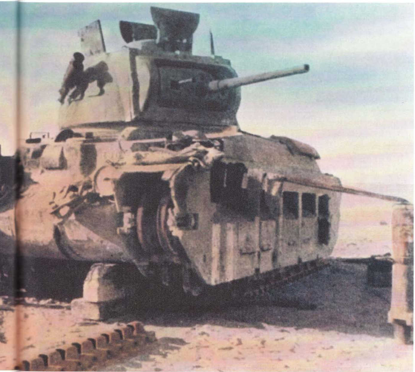
A desert casualty. This Matilda Mk II has had a track broken by enemy fire. Part of it is laid out in front of the tank which has some lumps of stone underneath to raise it off the ground. Behind is what appears to be a German heavy 4x4 cross-country car, which tends to suggest that the tank was captured while repairs were in progress. (Author's Collection)
