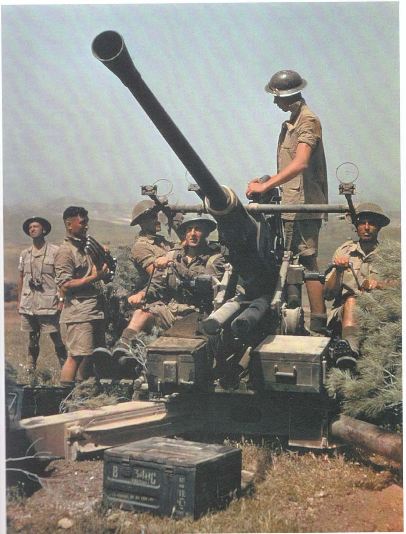
A Bofors light anti-aircraft gun crew in action on the Goubellat Plain near Tunis, May 1943. The Swedish-designed Bofors 40mm LAA gun was probably the best and most widely used of all LAA guns of the war. It was built under licence in the UK. (IWM — 920)
