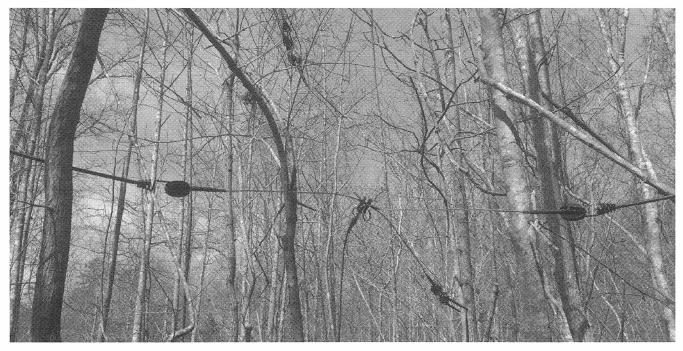
The Jungle Antenna's use is for creating the maximum amount of signal range from a fixed location. For sustainment communications purposes, this would be extremely useful for creating communications during the recovery phase of a natural disaster. This extends the RF range to roughly 6 miles. For tactical purposes, this radio would be in a fixed location at the TOC and for a receiving at a dedicated transmission site on a patrol as discussed in Chapter 6.
